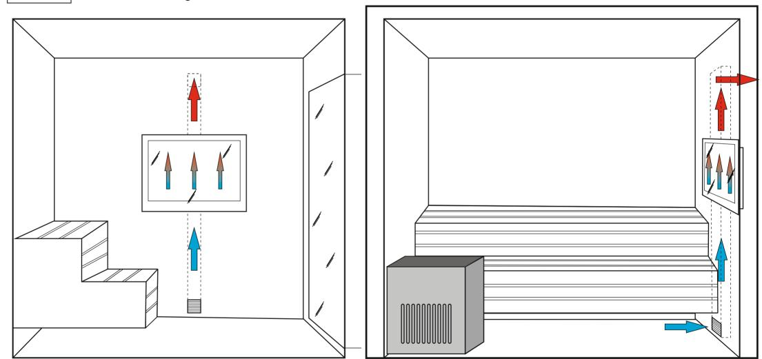
The ventilation duct shall deliver cool air to the middle-bottom part of the TV mounting box, and exhaust the heated up air from the middle of the top part. The ventilation duct cross-section is to be equivalent to at least 100 mm diameter tube.
